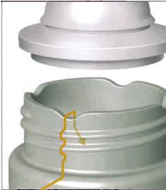
An inner skirt on the nipple, Pheil explains, hugs the inner diameter of the bottle neck and acts like a check valve, keeping the liquid in the bottle, while allowing the air to flow in to equalize the pressure.
